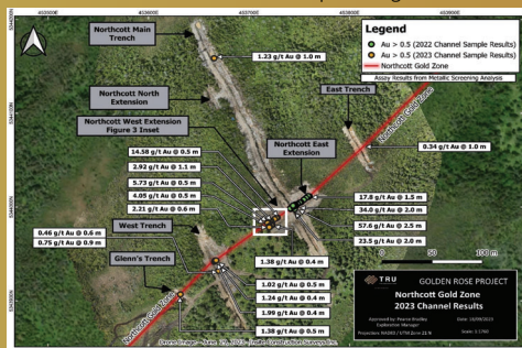
2022/2023 significant channel assay highlights from trenching, Northcott Gold Zone
