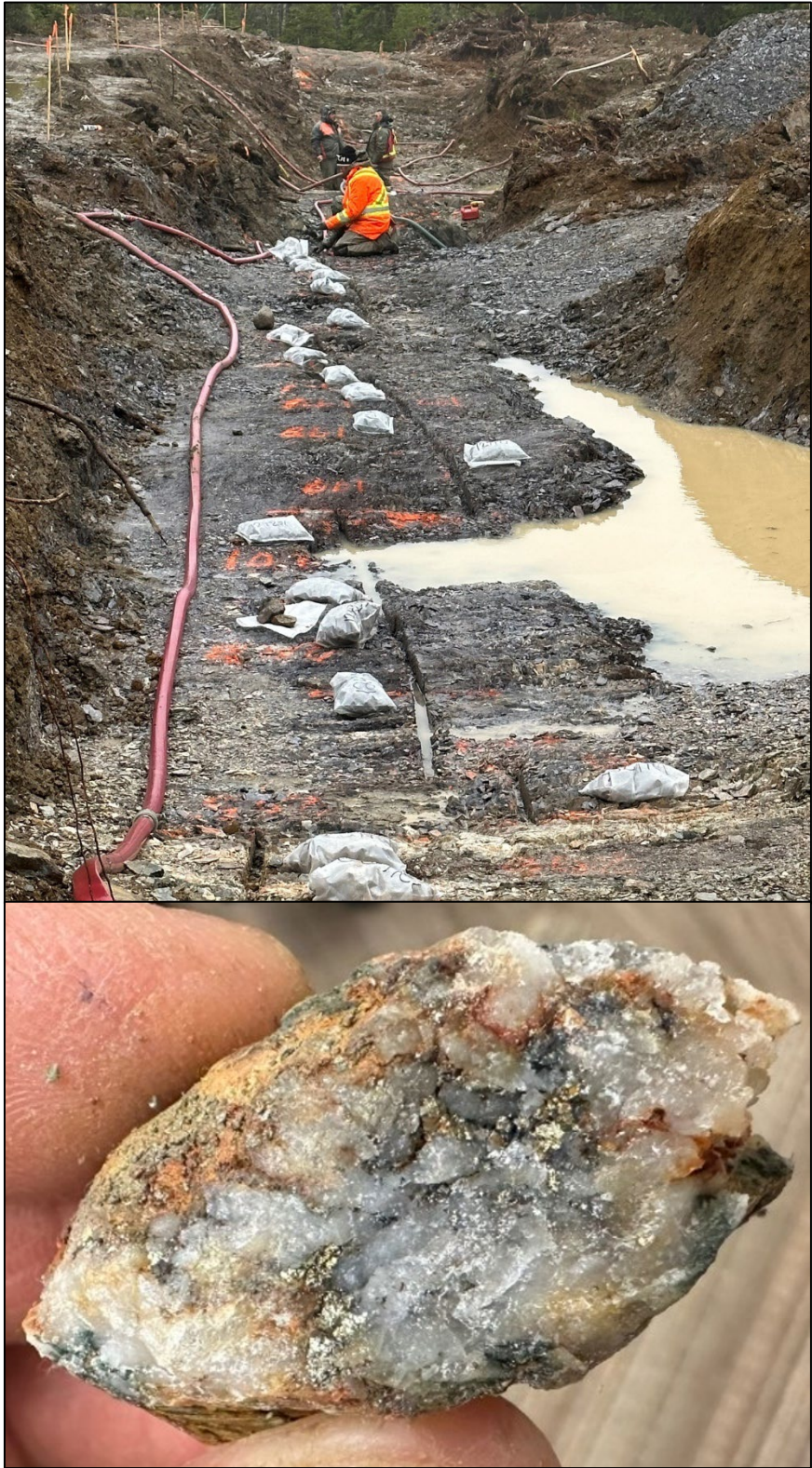
Figure 2: West Trench at Mark's Pond - mineralized quartz vein - containing abundant pyrite and chalcopyrite.
